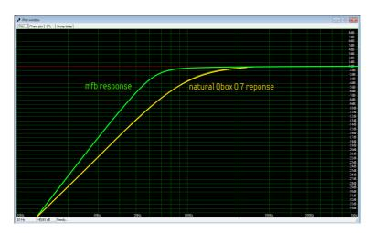
Example WINISD response plot for a driver with a F**c** of 60hz mounted in a sealed Q=0.7 enclosure with a natural F**box** of 120hz which is moved down to F**mfb** of 60hz.
