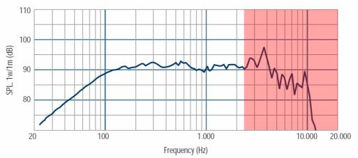
The third step is to decide on a low pass filter frequency - Flpf-using the drivers datasheet as reference. EVE's onboard lowpass filter follows a 2<sup>nd</sup> order Sallen Key setup, as such it is advised to choose Flpf at least 1 octave below the first occurrence of cone breakup. In the example above cone breakup happens in the red region onwards 2500hz making 1250hz or lower a valid choice for Flpf
