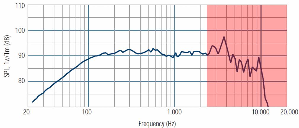
The third step is to decide on a low pass filter frequency -  $F_{lpf}$  - using the drivers datasheet as reference. EVE's onboard lowpass filter follows a 2<sup>nd</sup> order Sallen Key setup, as such it is advised to choose  $F_{lpf}$  at least 1 octave below the first occurrence of cone breakup. In the example above cone breakup happens in the red region onwards 2500hz making 1250hz or lower a valid choice for  $F_{lpf}$
