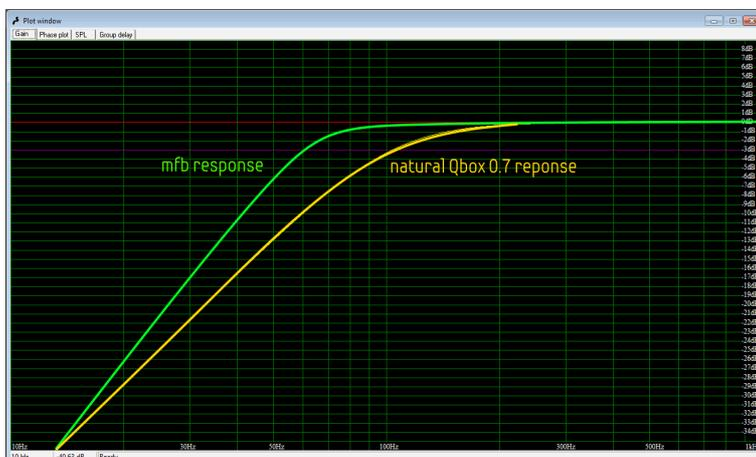
*Example WINISD response plot for a driver with a **Fc** of 60hz mounted in a sealed **Q=0.7** enclosure with a natural **Fbox** of 120hz which is moved down to **Fmfb** of 60hz.*
