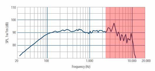
The third step is to decide on a low pass filter frequency - Fipf-using the drivers datasheet as reference. EVE's onboard lowpass filter follows a 2<sup>nd</sup> order Sallen Key setup, as such it is advised to choose Fipf at least 1 octave below the first occurrence of cone breakup. In the example below cone breakup happens in the red region onwards 2500hz making 1250hz or lower a valid choice for Fipf
