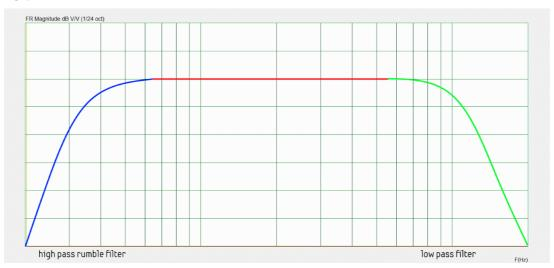
Build and tested EVE modules are preconfigured for a Rumble filter frequency of 32hz and a lowpass filter frequency of 493hz.
