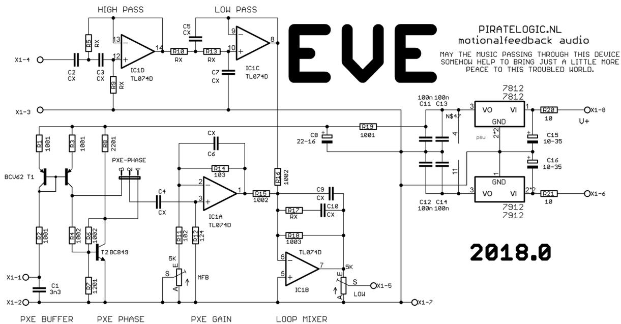
For a larger version of the schematics see page 11, the audio signal at X1-4 enters a second order high pass filter IC1D setting the lower bandwidth pole, the second order lowpass filter IC1C setting the upper bandwidth pole, refer to the **Crossover points** section for example filter values. It is advised to feed EVE at X1-4 from a low output impedance to avoid it from negatively affecting the hpf around IC1D.
