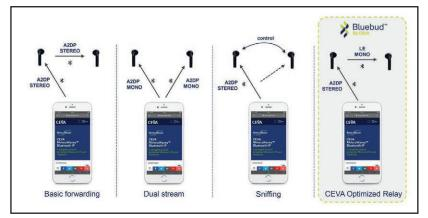
Different TWS Bluetooth connection approaches can be used to solve the "one source, two sinks" challenge of true wireless earbuds, including the new CEVA Optimized Relay mode.
