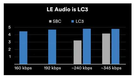
The new, high-quality, low-power Low Complexity Communications Codec (LC3) audio codec now part of LE Audio, enables product developers to make better design tradeoffs between key product attributes, such as audio quality and power consumption.
