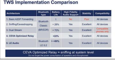
This chart shows the implementation comparison of true wireless stereo (TWS) products, including CEVA's latest Optimized Relay mode and the new Bluetooth LE Audio dual stream mode.
