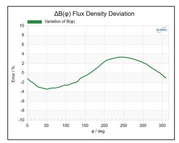
Figure 2: Deviation of the flux density of the magnetic field of the magnet used in the example transducer
