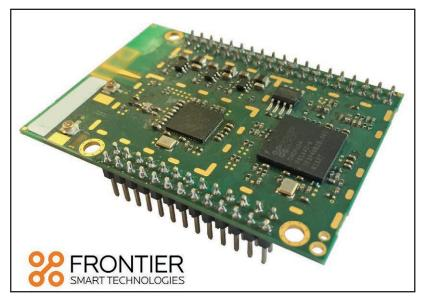
The latest Venice X platform from Frontier Smart Technologies is a high-quality SmartRadio module, supporting Bluetooth, FM, DAB+, and Internet connectivity via Wi-Fi.
