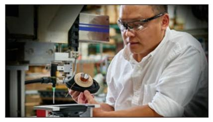
MISCO's speaker manufacturing uses robotics for precision adhesive placement.
