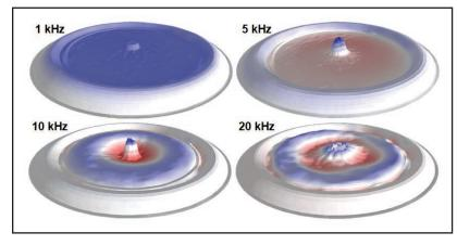
Figure 7: Example transducer measured near-field frequency response, direct sound response, and separated reflections
