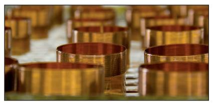
Eminence produces many of its voice coils in-house, including a wide range of voice coils with diameters from 1'' to 4''.
