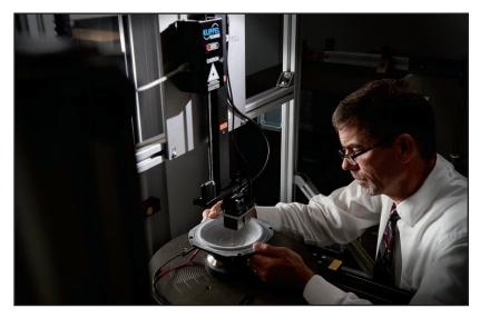
Klippel's Laser Scanner assists engineers in designing speaker cones and surrounds.
