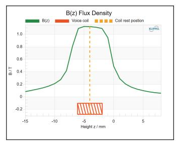
Figure 1: Flux density of the magnetic field of the magnet used in the example transducer
