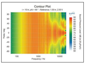
Figure 4: Example transducer horizontal plane contour plot
